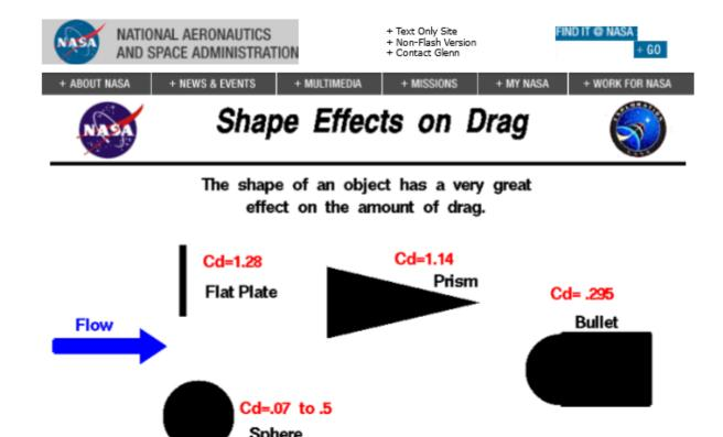
The <u>drag coefficient</u> is a number which engineers use to model all of the complex dependencies of <u>drag</u> on shape and <u>flow conditions</u>. The drag coefficient Cd is equal to the drag D divided by the quantity: <u>density</u> r times <u>reference area</u> A times one half of the <u>velocity</u> V squared.
